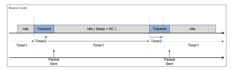
Figure 52. Beacon Mode Timing Diagram
