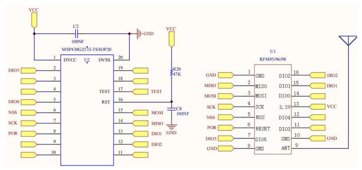
Figure 56:Reference Schematic
