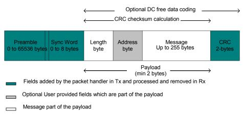
Figure 34. Variable Length Packet Format
