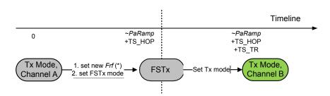
Figure 22. Transmitter Hopping
