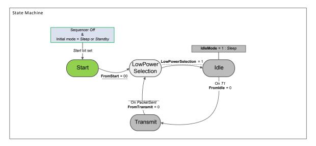
Figure 53. Beacon Mode State Machine
