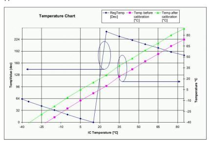
Figure 41. Temperature Sensor Response
