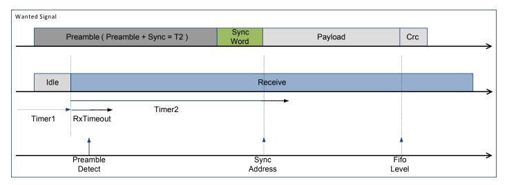
Figure 50. Listen Mode with Preamble Received & Valid SyncAddress
