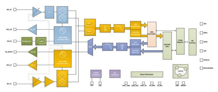
Figure 3. RFM95W/96W/98W Block Schematic Diagram
