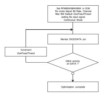
Figure 14. Floor Threshold Optimization
