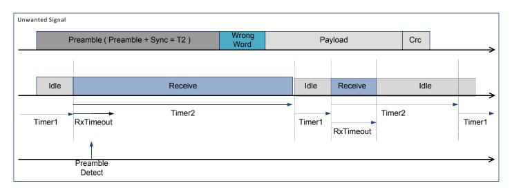
Figure 49. Listen Mode with Preamble Received and no SyncAddress
