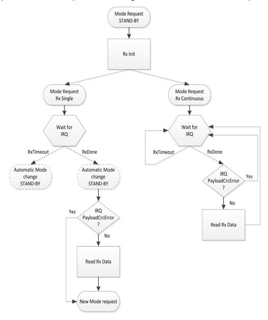
Figure 9. LoRa<sup>TM</sup> receive sequence.
