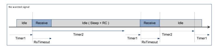
Figure 48. Listen Mode with no SyncAddress Detected
