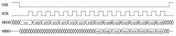
Figure 38. SPI Timing Diagram (single access)
