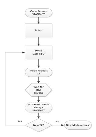
Figure 8. LoRa<sup>TM</sup> modulation transmission sequence.
