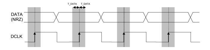
Figure 30. Tx Processing in Continuous Mode
