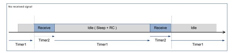
Figure 45. Listen Mode with No Preamble Received
