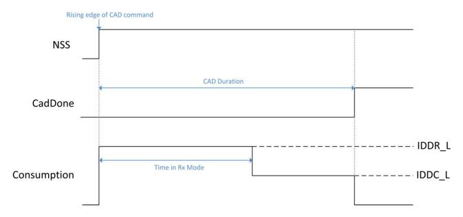
Figure 12. Consumption Profile of the LoRa CAD Process
