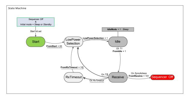
Figure 51. Wake On SyncAddress State Machine
