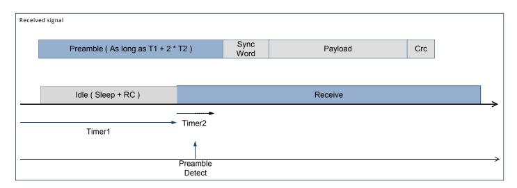
Figure 46. Listen Mode with Preamble Received
