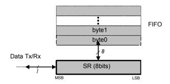
Figure 26. FIFO and Shift Register (SR)
