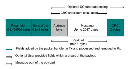
Figure 33. Fixed Length Packet Format
