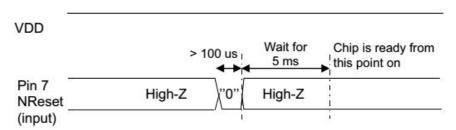
Figure 43. Manual Reset Timing Diagram
