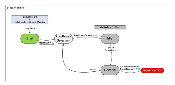
Figure 47. Wake On PreambleDetect State Machine
