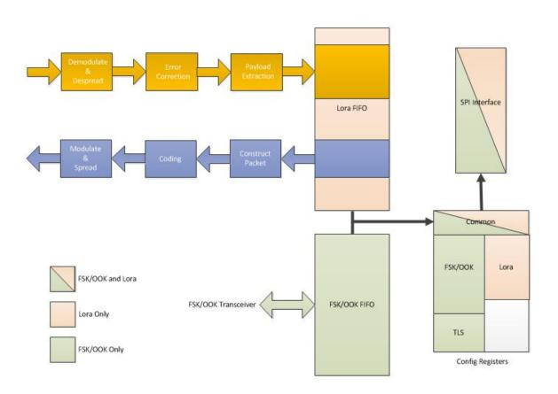
Figure 4. LoRa<sup>TM</sup> Modem Connectivity
