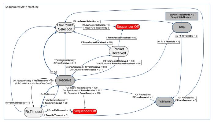
Figure 24. Sequencer State Machine
