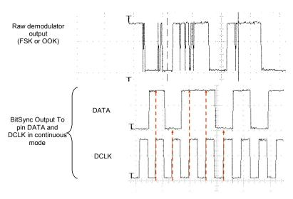
Figure 15. Bit Synchronizer Description
