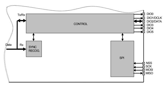
Figure 29. Continuous Mode Conceptual View
