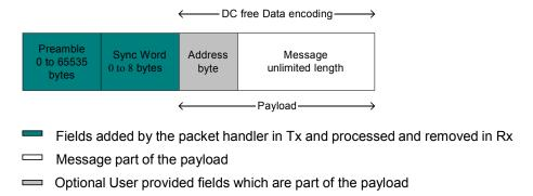
Figure 35. Unlimited Length Packet Format
