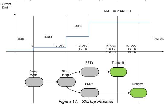
TS\_OSC is the startup time of the crystal oscillator which depends on the electrical characteristics of the crystal. TS\_FS is the startup time of the PLL including systematic calibration of the VCO.
