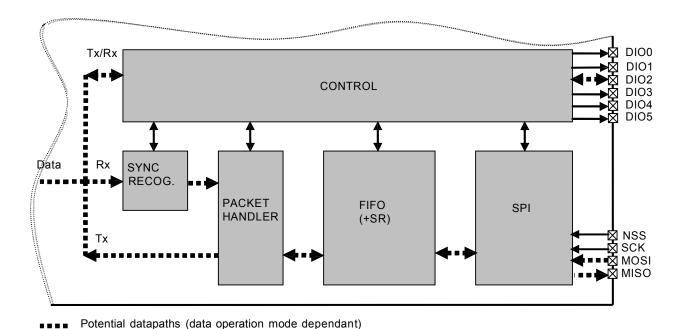
Figure 25. RFM95W/96W/98W Data Processing Conceptual View
