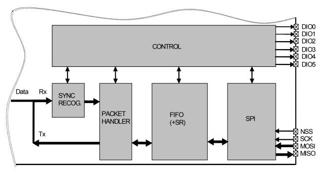
Figure 32. Packet Mode Conceptual View
