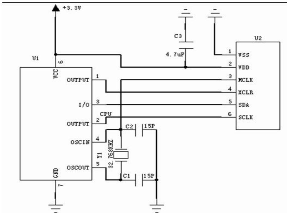
**Remark:** In the battery power supply product this application need be changed as: 32 KHz signal is outputted via the port of the MCU instead of the 32.768 KHz crystal to MCLK pin. The MCU will not output 32 KHz signal and keep low level when the HP01 enter to standby mode.
