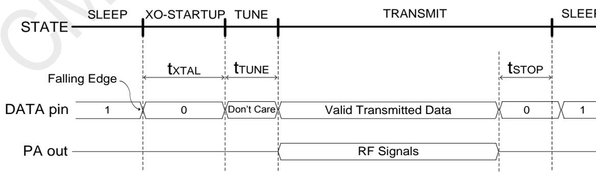
Figure 10. Transmission Enabled by DATA Pin Falling Edge
