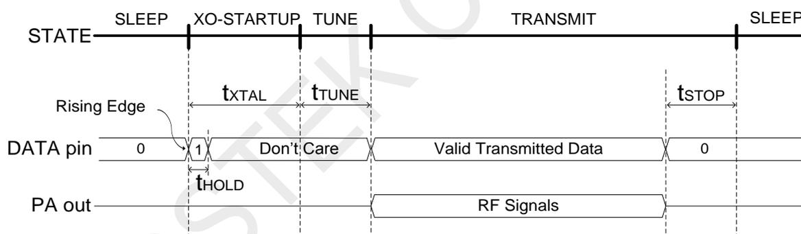
Figure 9. Transmission Enabled by DATA Pin Rising Edge
