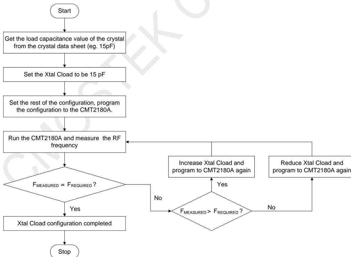
Figure 7. Procedure of Setting Xtal Clload
