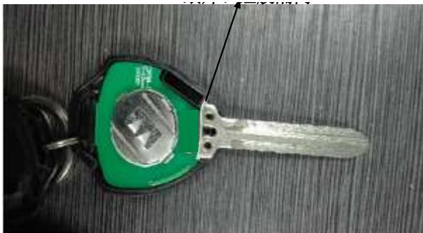
**Figure 5. Isolate Static Path of Inserted Metal**
