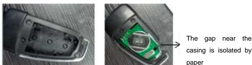
**Figure 4. Ensure Gaps Sealed Well**
