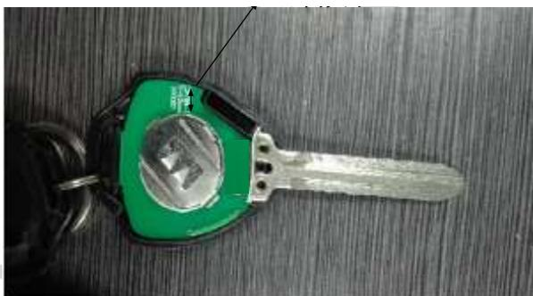
**Figure 6. Keep Distance between Internal Circuit and Edge of Structure**
