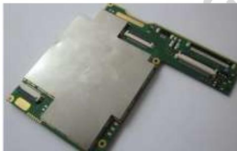
**Figure 8. Use Shield to Protect Electronic Circuit**
